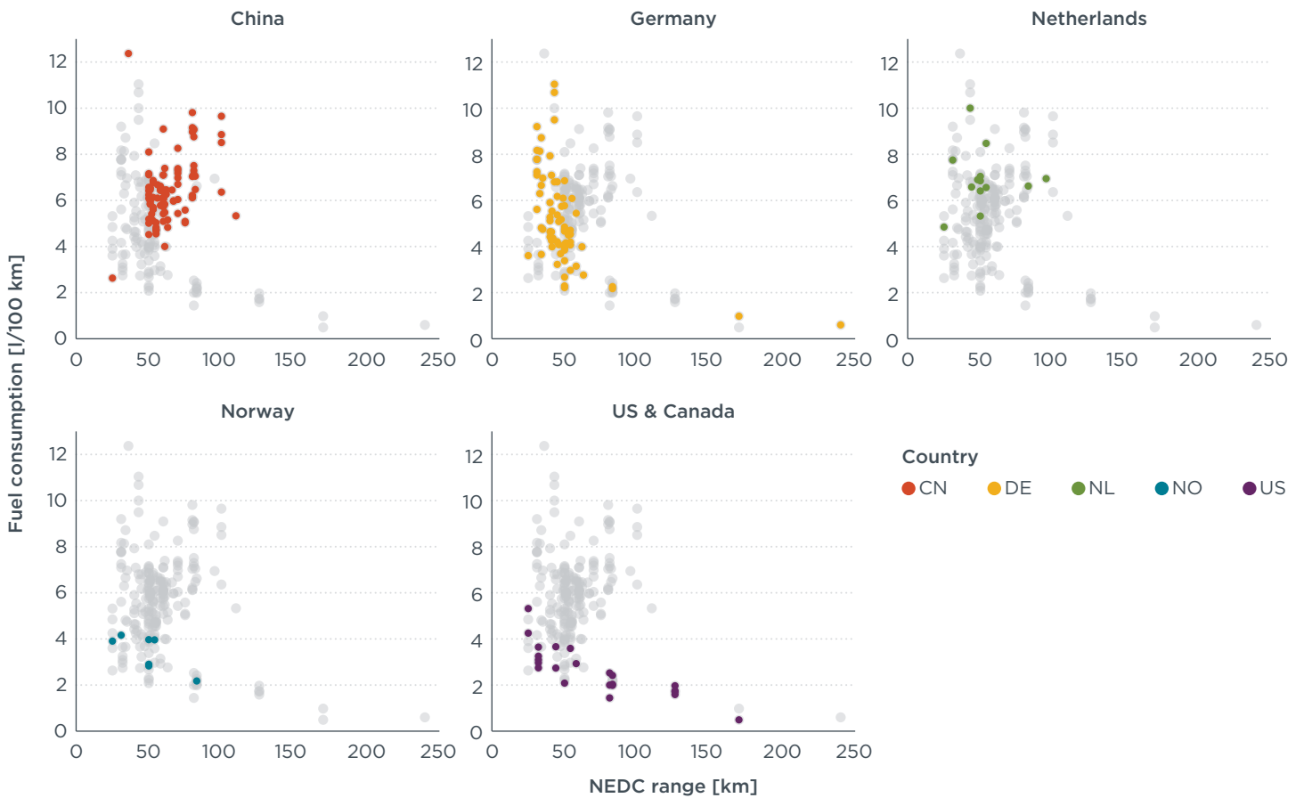
Figure 9. Fuel consumption by range and country. The average fuel consumption values of PHEV model variants are shown as colored circles. The grey dots are the full sample, and each small plot emphasizes the data from one country by country-specific color. The full sample of all countries and user groups is included.
